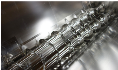
Dual Auger and Electropolished food contact surfaces
